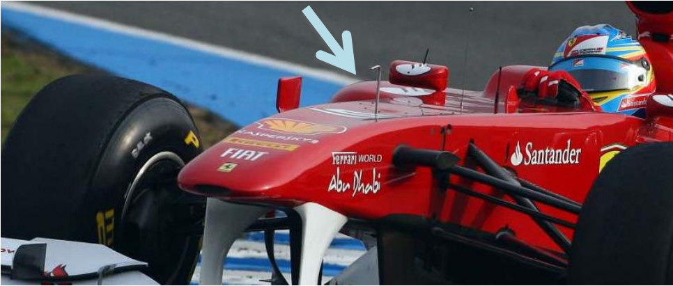
...with a Pitot Static Tube.
