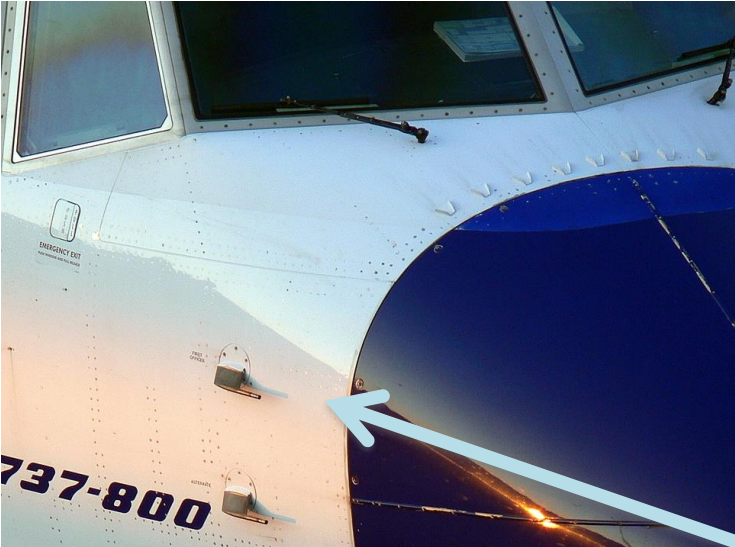
...with a Pitot Static Tube.
